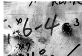
(d) Ti-6Al-4V solution treatment at 954°C and aged at 593°C in vacuum.
