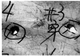
(b) Ti-15V-3Al-3Cr-3Sn annealed at 496°C .
