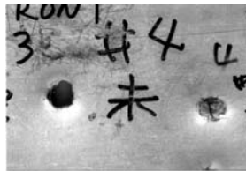
(d) Ti-6Al-4V solution treatment at 954°C and aged at 593°C in vacuum.
